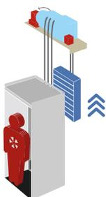
The same thing happens when the cabin goes up unloaded; in that case the counterweight is heavier, gravity moves it down and the motor generates energy again in the same way a dynamo does.
