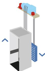
When the cabin goes down loaded, it weighs more than the counterweight so the cabin goes down by effect of gravity and the elevator motor acts as a brake, generating energy
